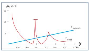
Impedance curves for network and filter
