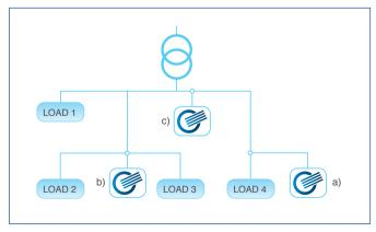
Figure 1: Installation of shunt capacitor banks
